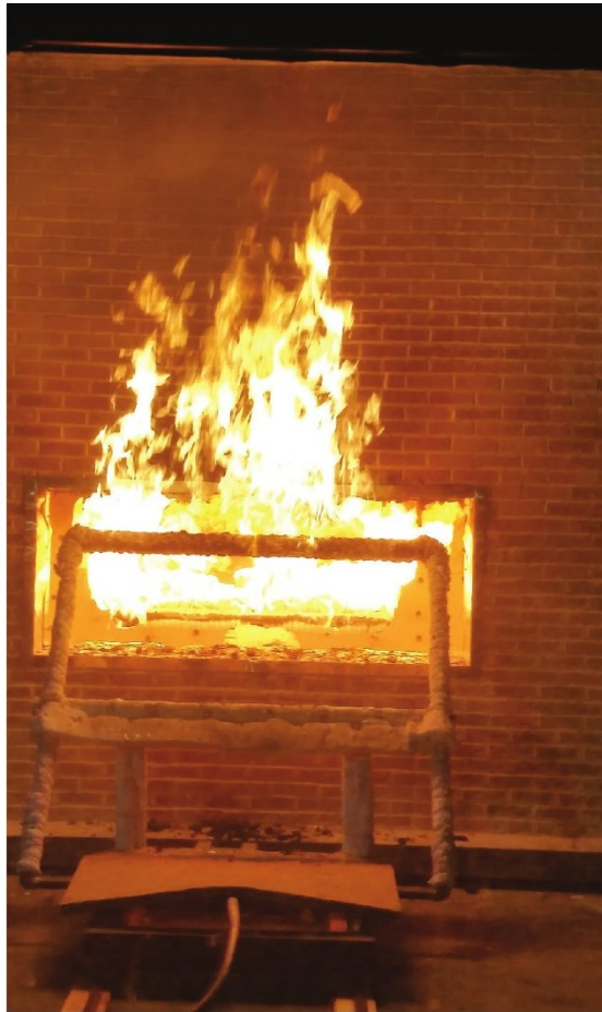
NFPA 285 test apparatus: Front view with the interior and window burners ignited and the exterior wall removed.
