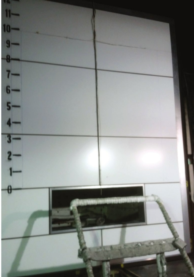
NFPA 285 test apparatus: Front view with window burner and exterior wall in place.
